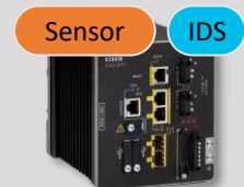
IC3000 Industrial Compute Hardware-Sensor DPI via SPAN to support brownfield
